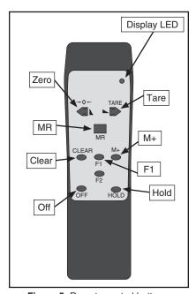
Figure 5. Remote control buttons.
